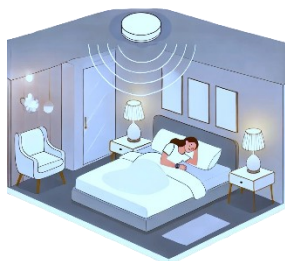
Fig. 1 Illustration of the Moonwalk study setup for non-contact sleep monitoring in a home environment using an overhead radar sensor (image source: https://samlab.org ).
